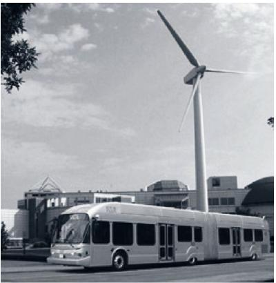
NASA's Glenn Research Center is designing a wind/sun-powered fueling system with zero carbon emissions for specially equipped city buses. An electrolyzer splits water molecules into oxygen and hydrogen, to be used for fuel cell-powered vehicles.
